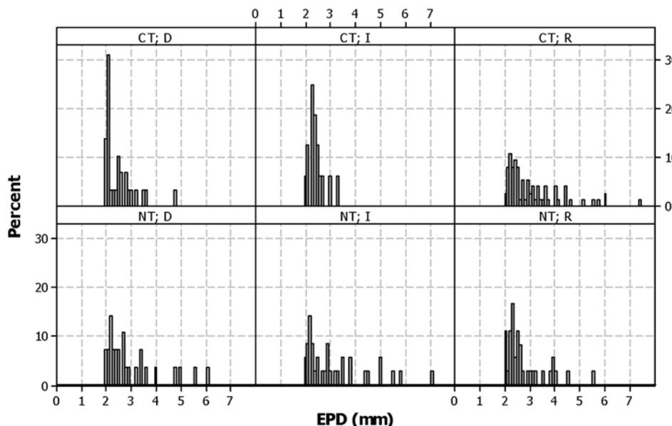
Fig. 2. Pore size distribution (PSD) of pores (equivalent pore diameter in the range  $2 > EPD > 7.5$  mm) of CT (conventional tillage) and NT (no-tillage) treatments, in different topsoil positions (D, 60 to 110 mm depth; I, drilling interrow; R, drilling-row, 0 to 60 mm).
