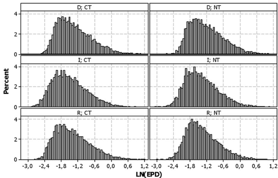
Fig. 1. Pore size distribution (PSD) of topsoil macropores from CT (conventional tillage) and NT (no-tillage) plots in three different topsoil positions (D, 60 to 110 mm depth; I, drilling interrow; R, drilling-row, 0 to 60 mm).
