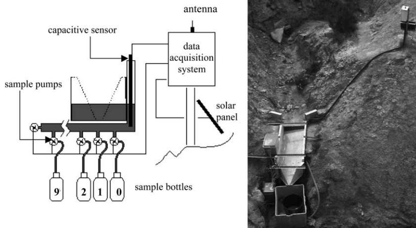
Fig. 2. H-flume gauging station in which a capacitive sensor records the height of water and an automatic pumping system samples runoff (with solutes and suspended sediment for further analysis). The data acquisition and transmission systems are also shown.
