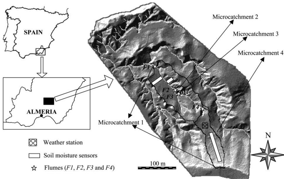
Fig. 1. The Cautivo field site (map compiled from a Digital Elevation Model at 1 m resolution), including the nested instrumented microcatchments, corresponding H-flumes (*F1*, *F2*, *F3* and *F4*), location of soil moisture probes and weather station.
