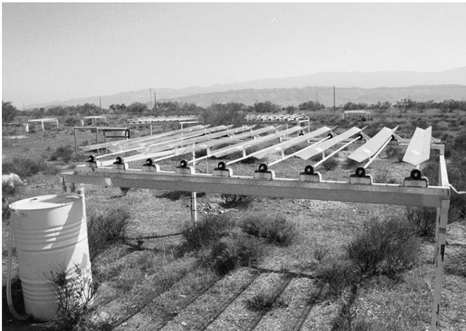
**Fig. 1.** An example of a rainout shelter installed in Tabernas (Almería, SE Spain). This rainout shelter belongs to MIX treatment during autumn. Polycarbonate bands are in position to intercept the rain.
